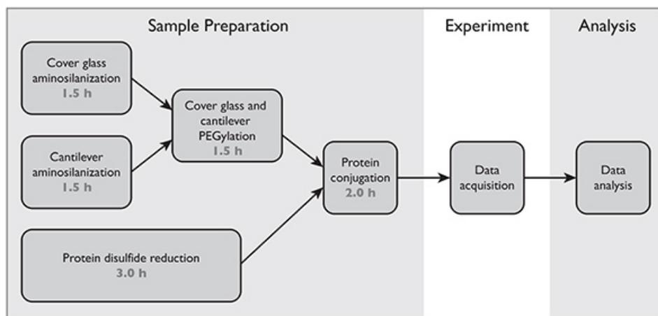
**Figure 2. Process flow diagram showing sample preparation steps followed by data acquisition and analysis.** [Click here to view larger image.](#)
