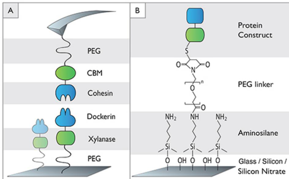
**Figure 1. Schematic of biomolecule immobilization.** (A) Xylanase-dockerin fusion proteins are attached to the glass slide via PEG linkers. The cantilever is similarly modified with a cohesin protein fused to a cellulose binding module (CBM). (B) Depiction of chemical bonding employed in cover glass and cantilever functionalization. [Click here to view larger image.](#)
