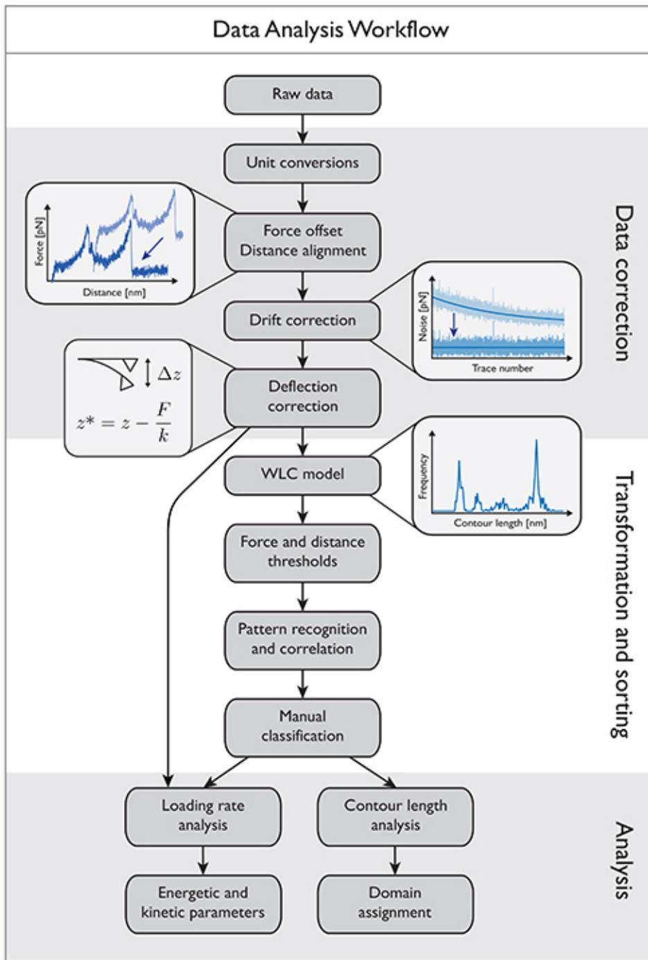
**Figure 3. Data analysis workflow diagram showing the processing steps involved in converting the raw detector signals into force-extension traces.** These traces are further analyzed to obtain information about receptor-ligand binding. The final results provide energetic and kinetic parameters about specific domains. [Click here to view larger image.](#)
