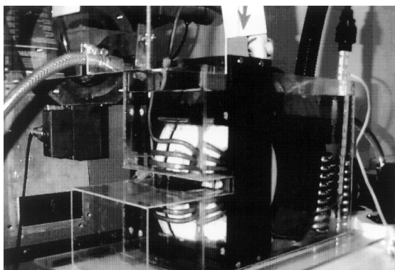
Fig. 2. Prototype applicator for regional AC magnetic field administration at a frequency of 500 kHz and field amplitudes of up to 10 kA/m. Depending on body cross-section and tissue conductivity lower frequencies should be used with humans, i.e. 50–100 kHz. The applicator site has a gap height of 20 mm, which is suitable for treating mice or other small animals.
